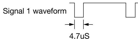
\*3 Measuring horizontal sync signal pull-in range
