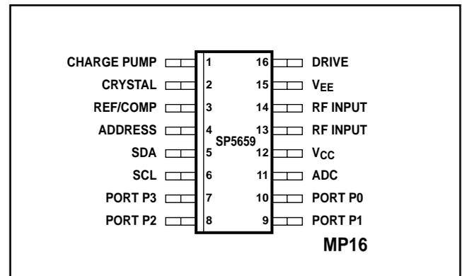
Figure 1 – Pin connections – top view
