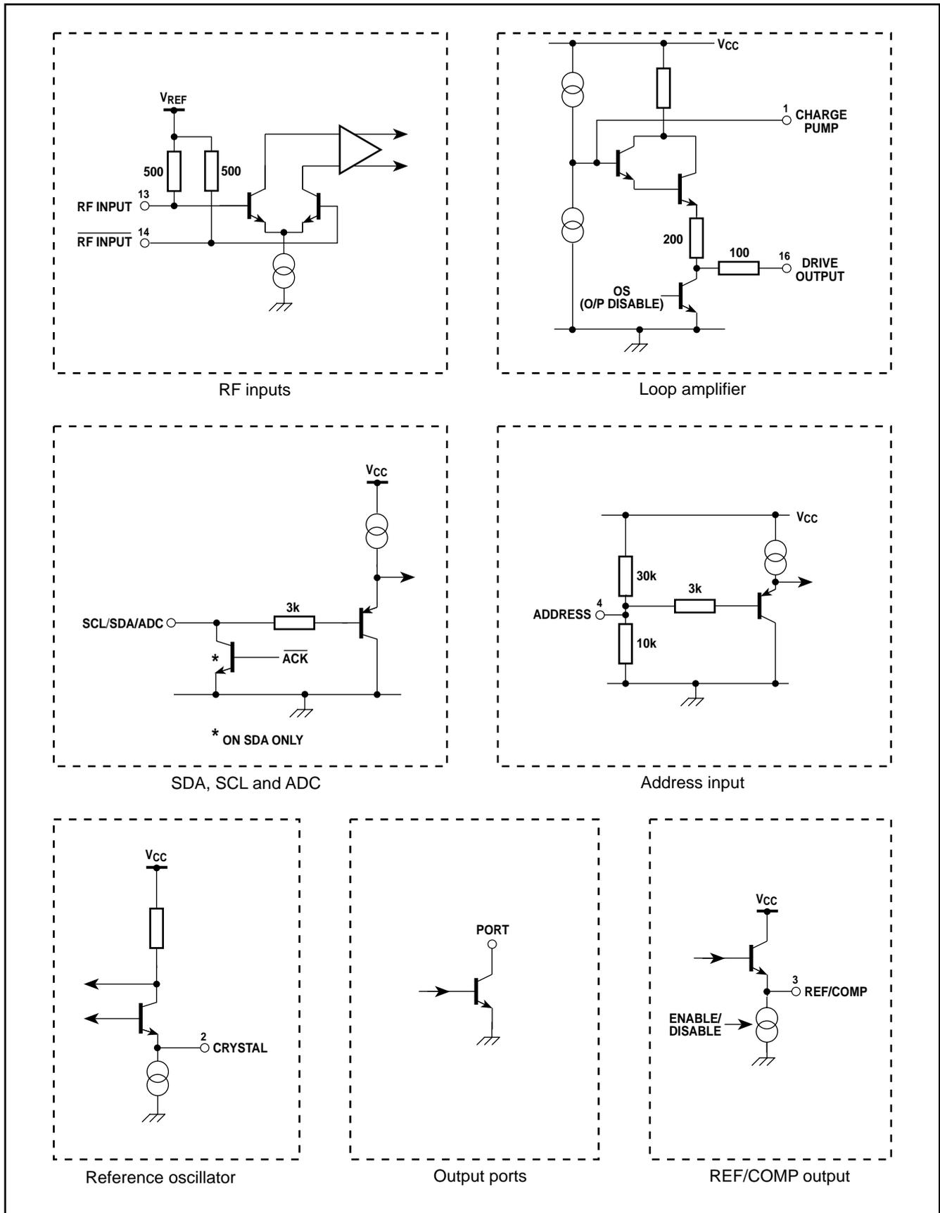
Figure 11 - Input/output interface circuits
