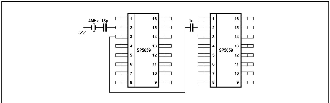
Figure 9 - Two SP5659 devices using a common reference
