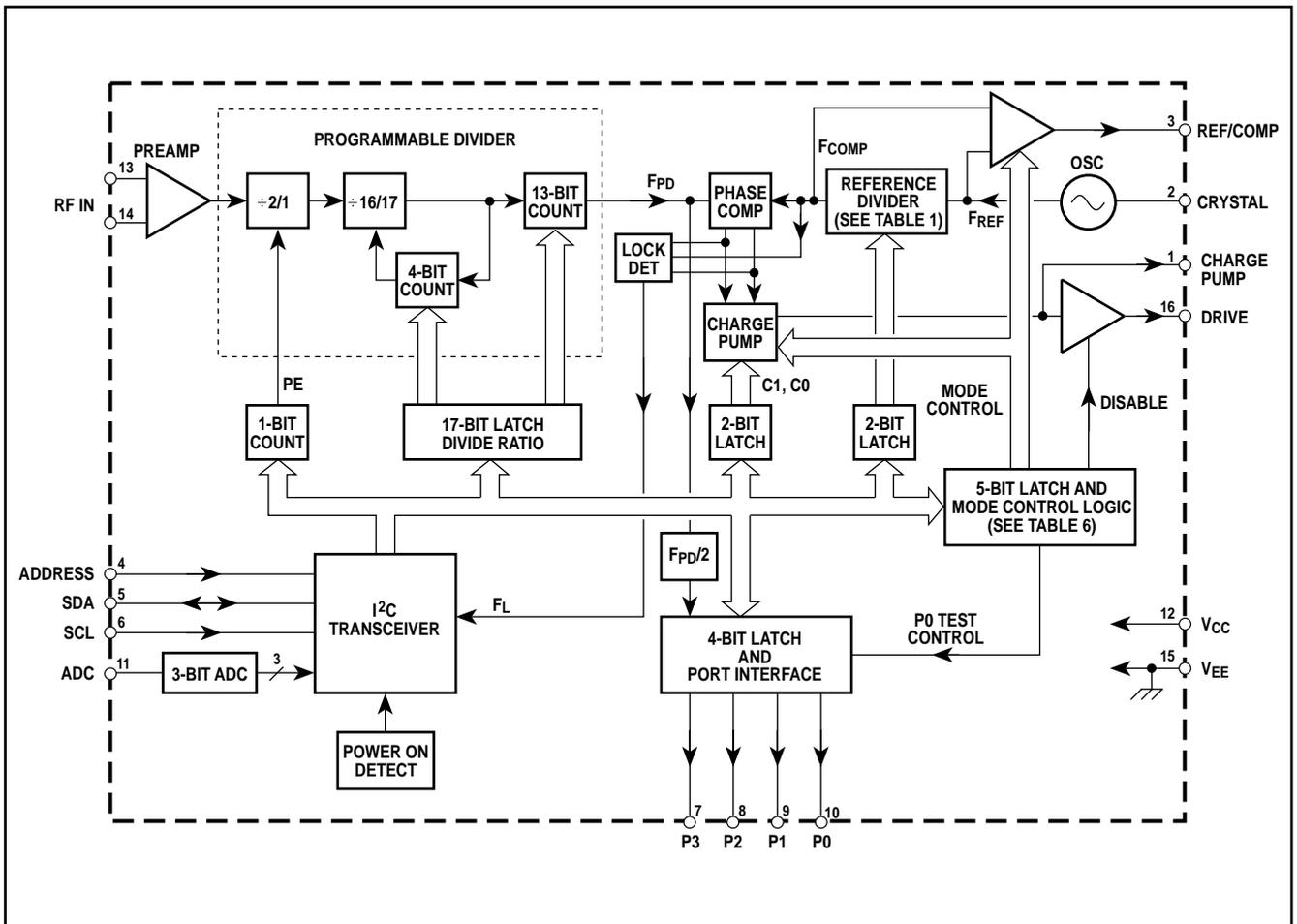
Figure 2 - Block diagram
