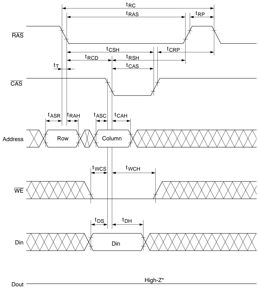
Delayed Write Cycle<sup>\*18</sup>
