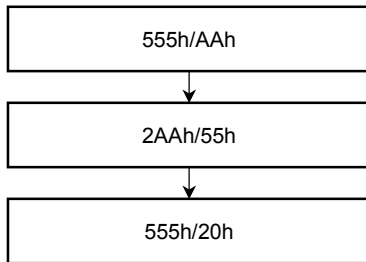
Fast Program Set Command Sequence (address/data)
