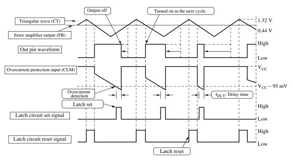
Figure 3. Waveforms of the pulse-by-pulse overcurrent protection operation
