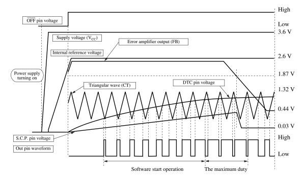
Figure 1. PWM comparator operation waveform
