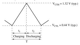
Figure 1. Triangular oscillation waveform
