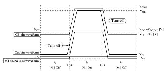
Figure 8. Bootstrap circuit operating waveform
