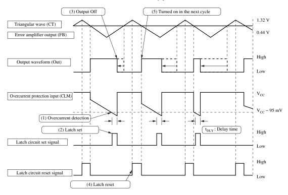
Figure 5. Waveforms of the pulse-by-pulse overcurrent protection operation
