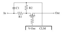
Figure 6. CLM noise filter circuit
