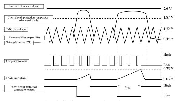
Figure 2. Short-circuit protection operation waveform
