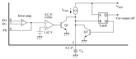
Figure 3. Short-circuit protection circuit
