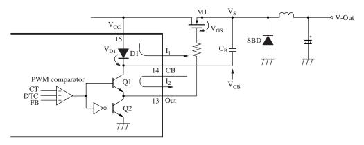
Figure 7. Bootstrap circuit of output block
