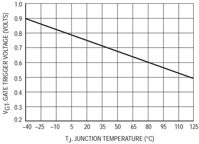
Figure 8. Typical Gate Trigger Voltage versus Junction Temperature
