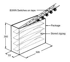
Do not press strongly, vibrate, or drop the package, otherwise the terminals of the Switches may deform.
