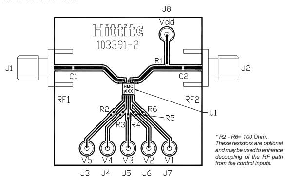
The circuit board used in the final application should use RF circuit design techniques. Signal lines should have 50 ohm impedance while the package ground leads should be connected directly to the ground plane similar to that shown. A sufficient number of via holes should be used to connect the top and bottom ground planes. The evaluation circuit board shown is available from Hittite upon request.
