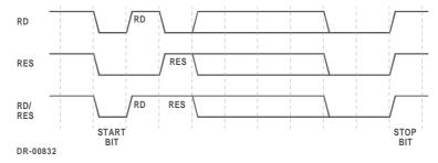
Read, Reset and Read/Reset of integrator for reactive energy
