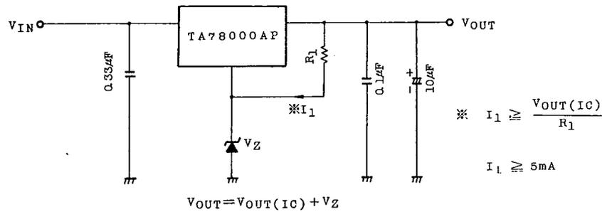
(b) Voltage boost by use of resistor
