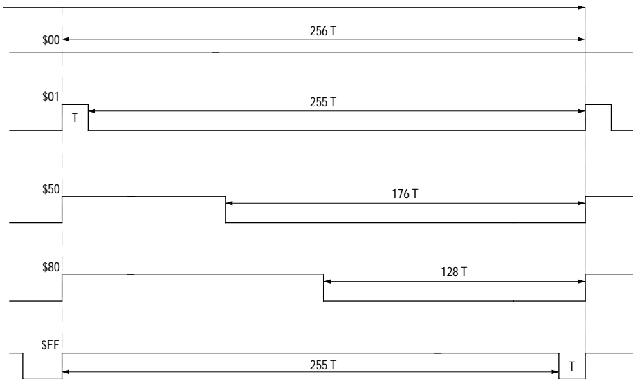
Figure 12-2 PWM output waveforms (POL = 1, active high)
