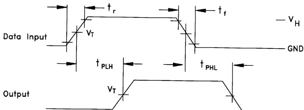
Input and output threshold voltage:
