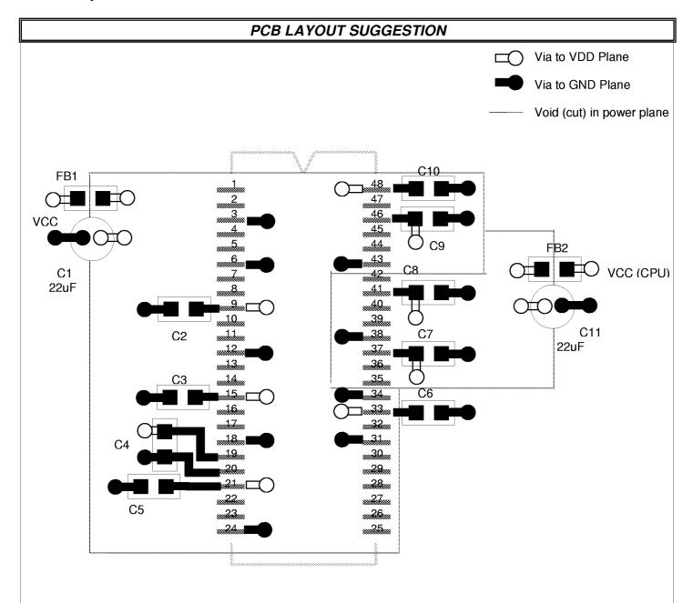
This is only a layout recommendation for best performance and lower EMI. The designer may choose a different approach but C2, C3, C4, C5, C6, C7, C8, C9, and C10 (all are 0.1 uf) should always be used and placed as close to their VDD pins as is physically possible. The topological hookup of C4 with respect to its power and ground vias is especially important.
