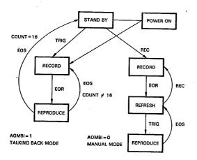
REC = RECIN pin is triggered TRIG = TRIG pin is triggered EOR = End Of Record EOS = End Of Speech
