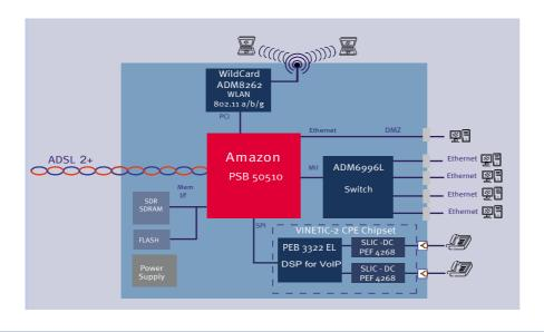
ADSL2/2+ SOHO Gateway with WLAN and VoIP Application Example
