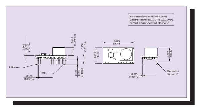
Figure 1: Mechanical Drawing - Horizontal Mount Version
