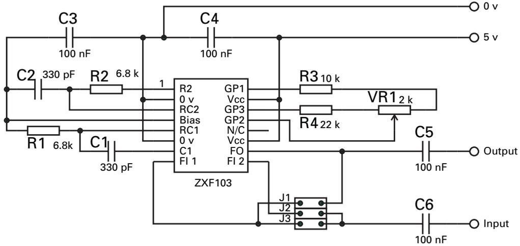
The evaluation board is designed for operation at 70kHz.
