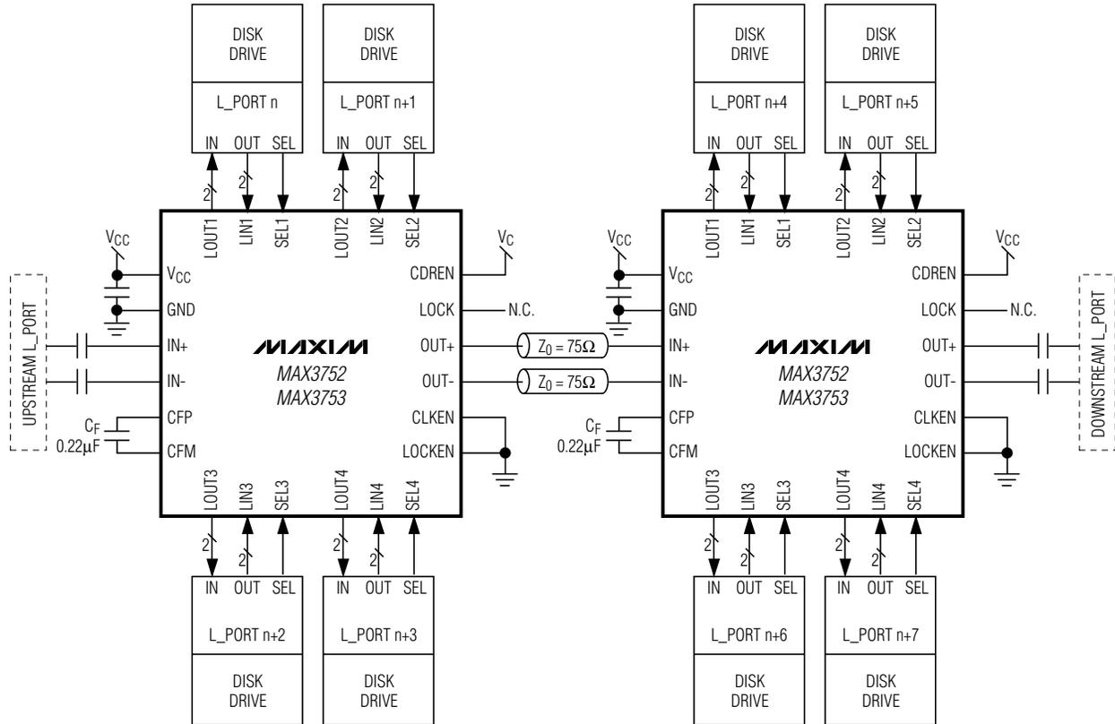
**NOTE:** ALL HIGH-SPEED INPUTS AND OUTPUTS (IN±, OUT±, LIN±, AND LOU±) SHOULD BE CONNECTED USING CONTROLLED IMPEDANCE TRANSMISSION LINES. AC-COUPLING MAY ALSO BE REQUIRED. ALL CAPACITORS ARE 0.1μF UNLESS OTHERWISE INDICATED.
