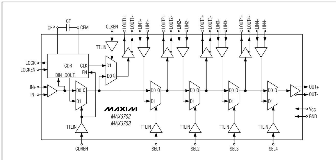
Figure 1. Functional Diagram
