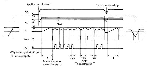
Note : Edge-triggered at the point indicated by the arrow of  $C_{\mbox{\scriptsize K}}$  signal.
