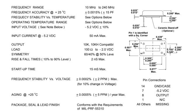
NOTE: For PECL applications, Xsis 300 Series ECL oscillators can be operated with +5 VDC ± 10% on Pin 14 and power supply return on Pin 7. The output logic levels will still be referenced to +5 VDCand the case will be at +5 VDC, however, 0.8 V peak to peak output signal can be AC or DC coupled as necessary.
