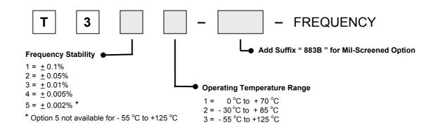
EXAMPLE: T343 - 883B - 24.000 MHz = 4 Pin Package, 10KH ECL, ± 0.005% over -55 °C to +125 °C, Mil-Screened, and 24.000 MHz
