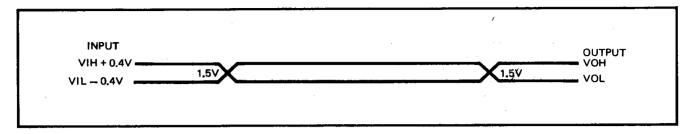
A.C. Testing: All input signals (other than CLK) must switch between VIL -0.4V and VIH +0.4V. CLK must switch between 0.4V and 3.9V.  $T_{\rm R}$  and  $T_{\rm F}$  must be less than or equal to 15ns.
