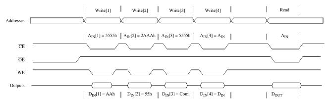
For all waveforms,  $A_{IN[4:1]}$ , and  $D_{IN[4:1]}$  = Address and Data for write cycles 1–4;  $D_{IN}$  = Data to be programmed at address  $A_{IN}$ ; Com. = Command byte input on the DQ pins during Write<sub>[3]</sub>;  $D_{OUT}$  = Status byte, Manufacturer ID code, or array data for verify.
