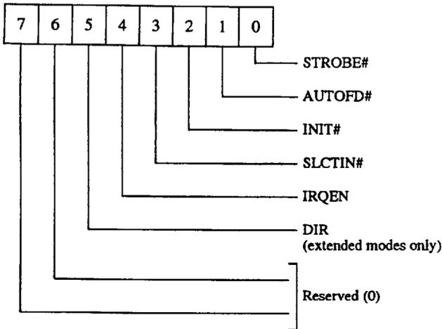
The parallel port Data Control Register (DCR) provides all output control signals to the printer.
