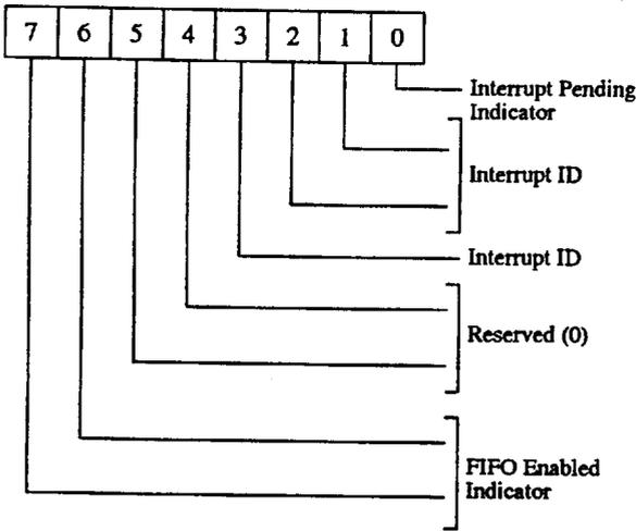
To provide minimum software overhead during data character transfers, the UART prioritizes interrupts into four levels and records these in the Interrupt Identification Register (IIR). The four levels of interrupt conditions in order of priority are
