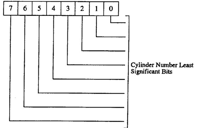
This register contains the eight least significant bits (LSB) of the desired cylinder number.
