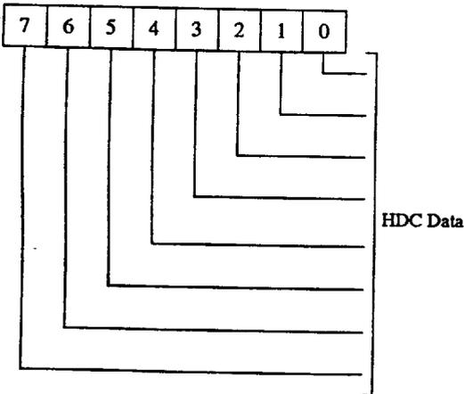
The data register provides an 8 or 16-bit data path to the IDE disk drive. This register handles all data transfers between the host and the hard disk.
