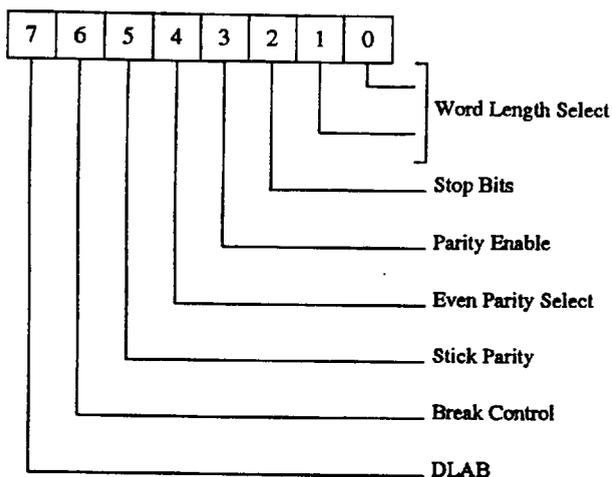
The Line Control Register (LCR) is used to specify the format of the asynchronous data communications exchange and to set the divisor latch access bit.
