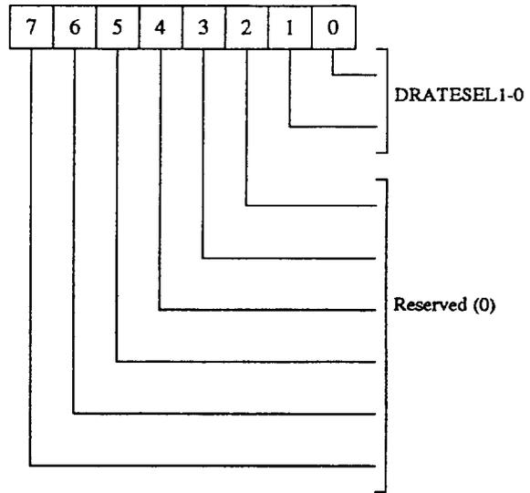
The Configuration Control Register (CCR) sets the data rate. This register is not affected by a software reset and defaults to 250Kb/s on a hardware reset. The data rate of the FDC is determined by the last write to either the configuration control register or the data rate select register.
