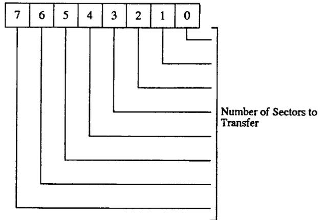
This register contains the number of sectors to be transferred during a VERIFY, READ, WRITE, or FORMAT command (see "FDC Command Set" for command descriptions). A 0 value means a 256 sector transfer.
