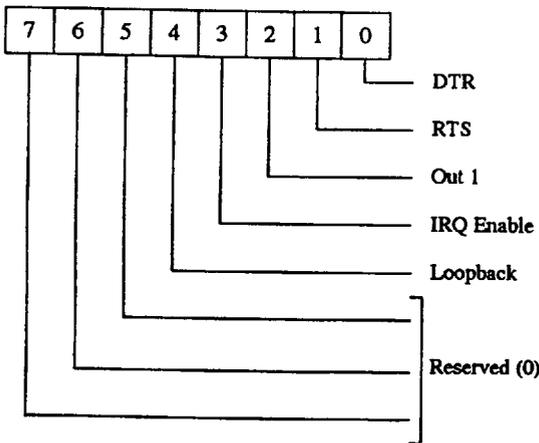
This register controls the interface with the modem, data set, or peripheral device emulating a modem.
