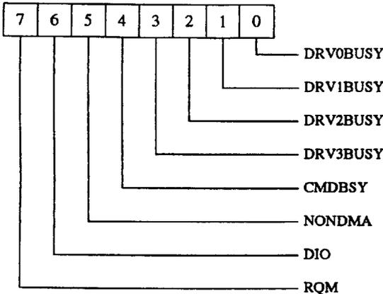
The Main Status Register (MSR) is always available to be read. The MSR is used for controlling command input and result output for all commands. It gives the current status of the FDC, and indicates when the disk controller is ready to send or receive data through the data register (FIFO).
