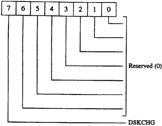
When the Digital Input Register (DIR) is in PC/AT mode, only bit 7 (DSKCHG) is driven. Bits 6-0 are tristated to avoid conflict with the fixed disk status register at the same address. The DSKCHG bit monitors the pin of the same name and reflects the opposite value seen on the disk cable. Bit 7 is forced inactive along with the inputs from the floppy drive, while the other bits remain tristated. The Digital Input Register is unaffected by a software reset.
