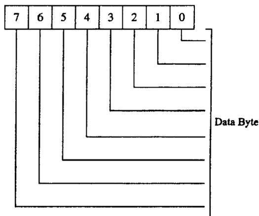
This register holds the incoming data byte. Bit 0, the Least Significant Bit (LSB), is received first. The data is initially assembled in the Receiver Shift Register (not user accessible) before it is loaded into the Receive Buffer or Receiver FIFO.
