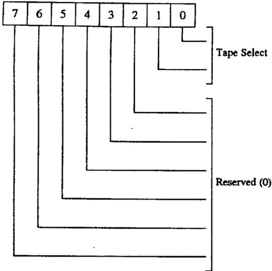
The Tape Drive Register (TDR) is included for software compatibility. The 82C733 digital data separator does not have to be modified for tape support. The contents of this register are not internal to the device.
