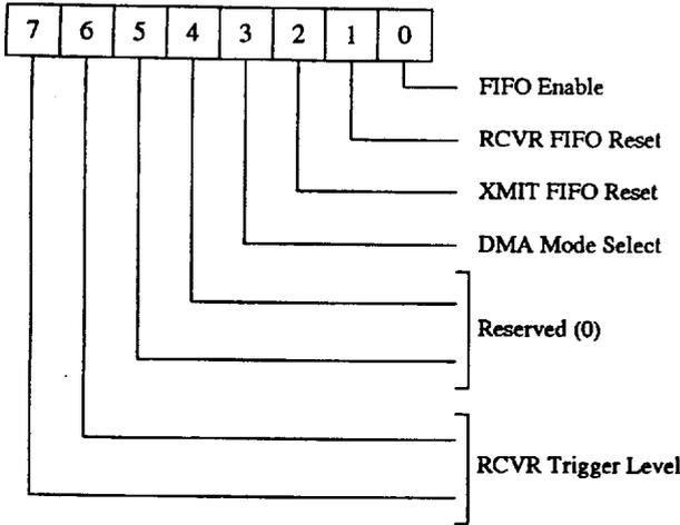
This write-only register is at the same location as the Interrupt Identification Register, a read-only register. The FIFO Control Register is used to enable the FIFOs, clear the FIFOs, set the RCVR FIFO trigger level, and select the type of DMA signaling
