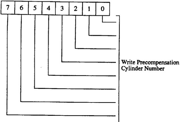
This register is written to by the host. It usually contains the number of the cylinder where the write precompensation is to be used.
