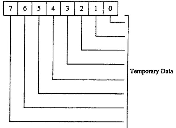
The MCR shows the current state of the control lines from the modem or peripheral device to the CPU. Four of the bits provide change data. These bits are set to 1 when a control input from the modem changes state, and are reset to 0 when the CPU reads the MSR.
