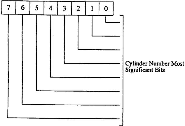
This register contains the eight most significant bits (MSB) of the desired cylinder number.
