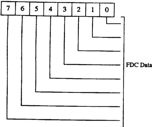
All command/status parameter information and disk data transfers go through the Data Register or FIFO. The data transfers are controlled by bits D7 (RQM) and D6 (DIO) in the Main Status Register. The FIFO is 16 bytes and has programmable threshold values.
