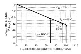
**Reference Short Circuit Current vs. Temperature**
