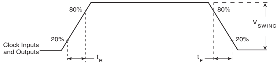
FIGURE 5 - INPUT AND OUTPUT RISE AND FALL TIME
