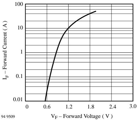
Figure 3. Typ. Forward Current vs. Forward Voltage
