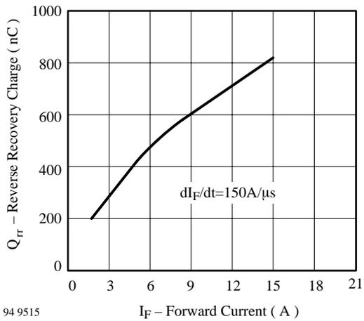
Figure 4. Reverse Recovery Charge vs. Forward Current
