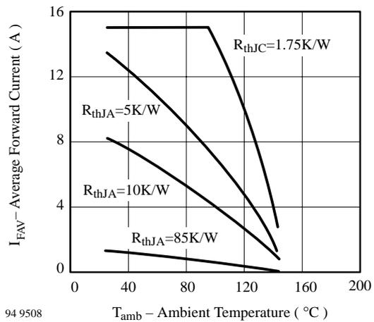
Figure 2. Max. Average Forward Current vs. Ambient Temperature
