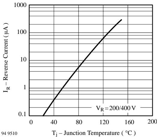
Figure 1. Typ. Reverse Current vs. Junction Temperature
