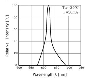
Fig. 5 Radiation Diagram
