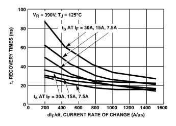
FIGURE 4. ta AND tb CURVES vs dlF/dt
