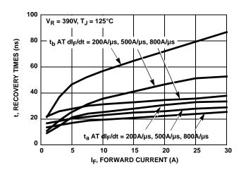
FIGURE 3. ta AND tb CURVES vs FORWARD CURRENT
