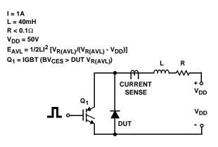
FIGURE 13. AVALANCHE ENERGY TEST CIRCUIT
