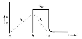
FIGURE 14. AVALANCHE CURRENT AND VOLTAGE WAVEFORMS
