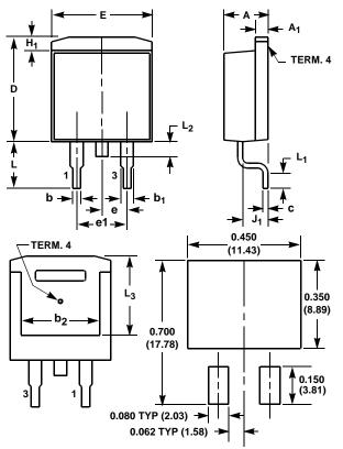
MINIMUM PAD SIZE RECOMMENDED FOR SURFACE-MOUNTED APPLICATIONS
