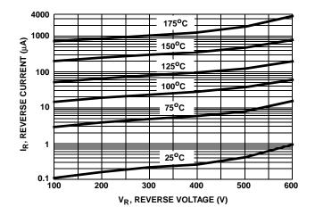
FIGURE 2. REVERSE CURRENT vs REVERSE VOLTAGE
