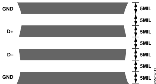
Figure 22. Typical Arrangement of Signal Tracks
