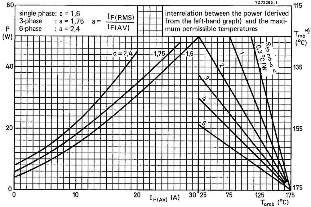
\*)  $T_{mb}$ -scale is for comparison purposes only and is correct only for  $R_{th\ mb-a} \leq 6,5\ ^\circ\text{C}/\text{W}$
