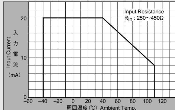
Note : R<sub>in</sub> of Hall element decreases rapidly as ambient temperature increases. Ensure compliance with input current derating curve envelope, throughout the operating temperature range.
