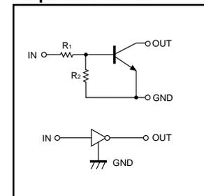
$R_1=4.7\text{k}\Omega / R_2=4.7\text{k}\Omega$
