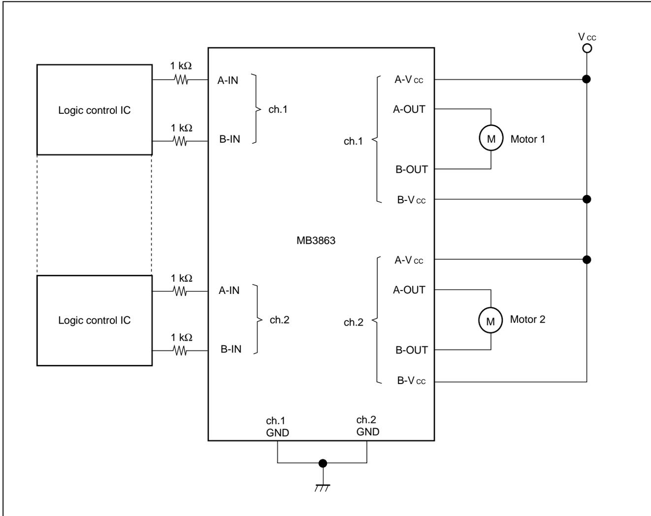
Note : If input voltage is applied when power is not supplied, over-current flows into the device via the input pins. In this case, connect a resistor of at least 1 kΩ in series with the input pins to prevent passage of a large current.
