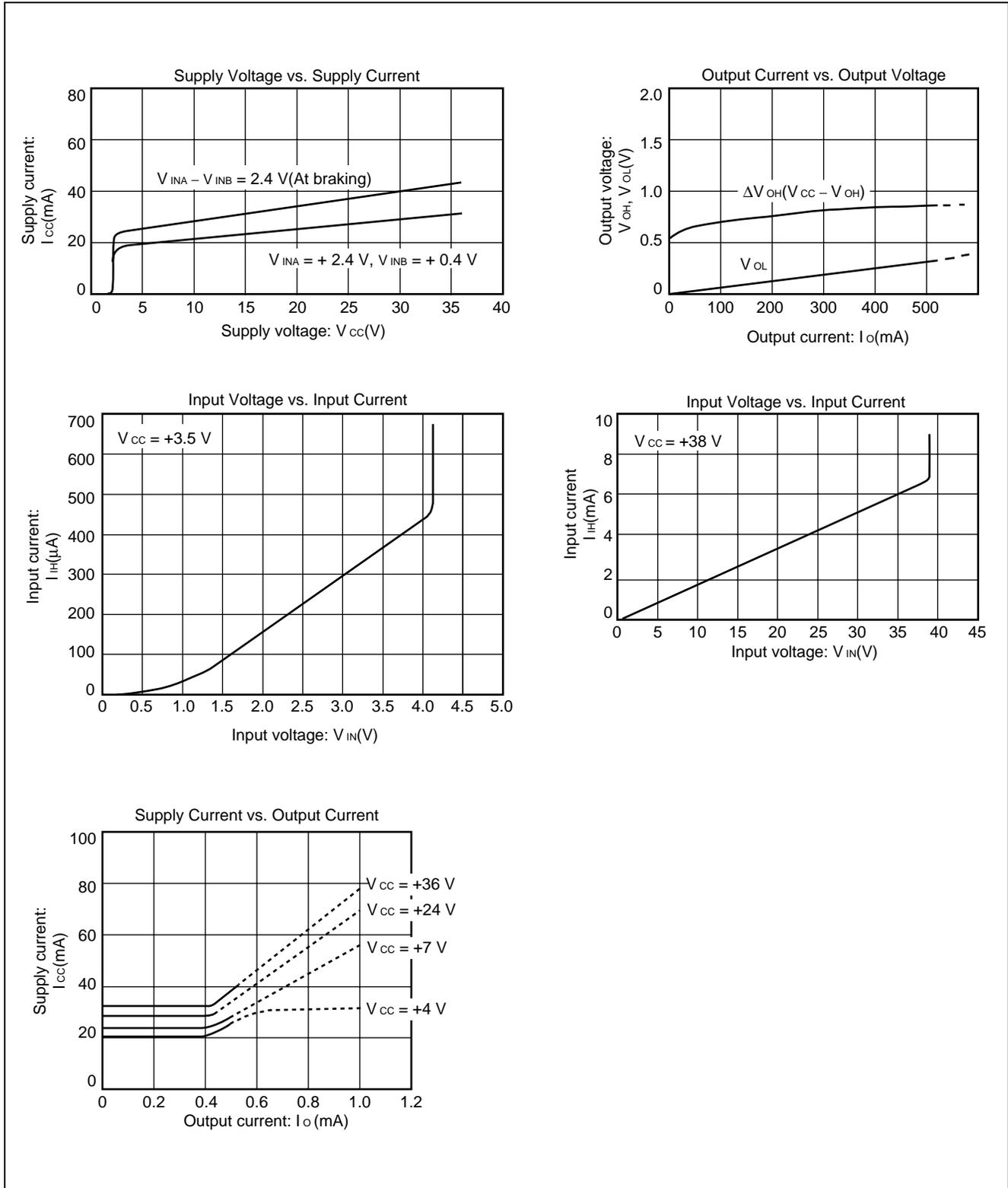
Note : The above characteristic curves are at  $T_a = +25^\circ\text{C}$
