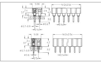
Straight receptacle: solder tail, double row, low profile h = 4.2 mm
