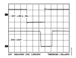
Figure 17. Propagation Delay Timing 100 mV Overdrive
