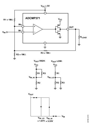
Figure 20. Noninverting Comparator Configuration with Hysteresis
