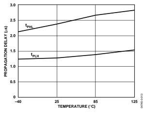
Figure 7. Propagation Delay vs. Temperature
