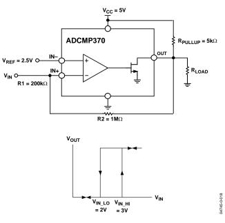
Figure 19. Noninverting Comparator Configuration with Hysteresis
