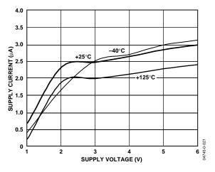
Figure 8. Supply Current vs. Supply Voltage (Output Low)
