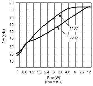
FIG.4 The relation curve between  $f_{\text{SW}}$  and output power  $P_{\text{OUT}}$
