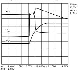
Startup Behavior At Nominal Load Condition V<sub>DCIN</sub>=350 V
