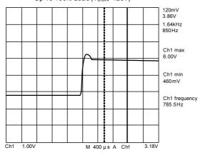
Feedback Voltage During Loadjump From10% Up To 100% Load ( $V_{DCIN}$ =350V)
