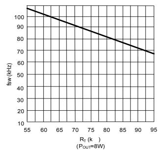
FIG.5 The relation curve between f<sub>SW</sub> and R<sub>T</sub>
