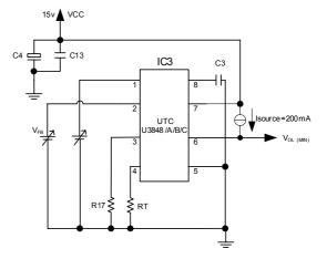
FIG.11 driver test circuit with source current
