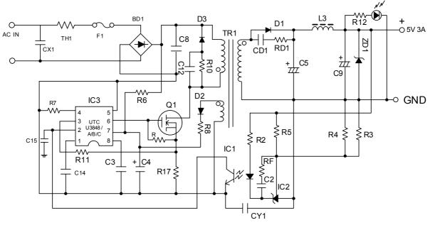
FIG.12 U3848/A/B/C Typical Application Circuit
