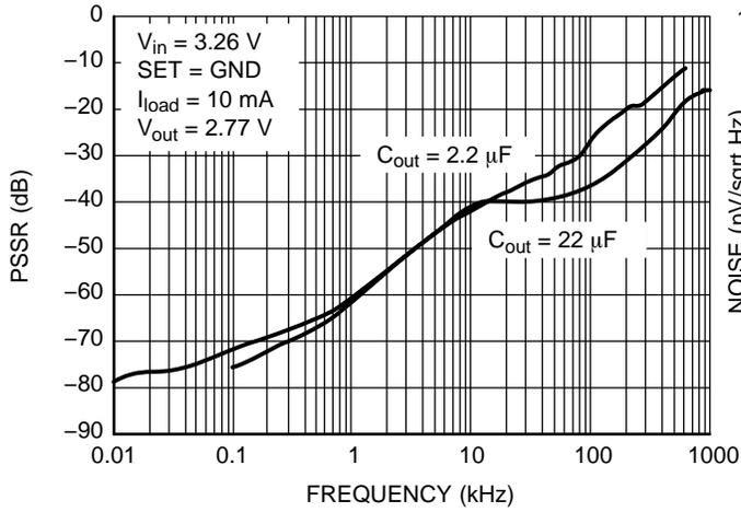
Figure 7. Power Supply Rejection Ratio
