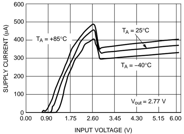
**Figure 4. No Load Supply Current vs. Input Voltage**
