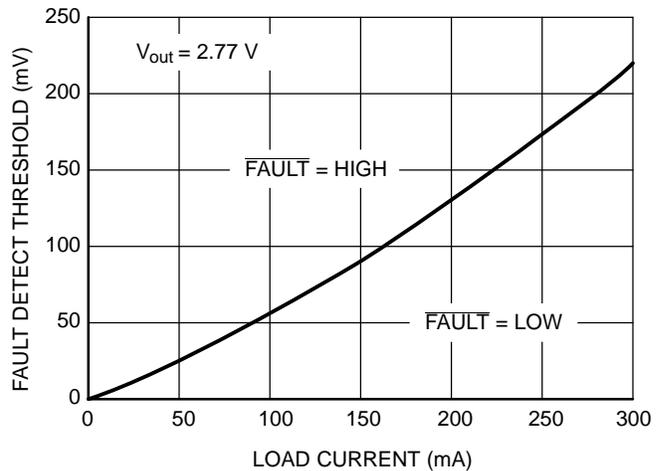
**Figure 6. Fault Detect Threshold vs. Load Current**
