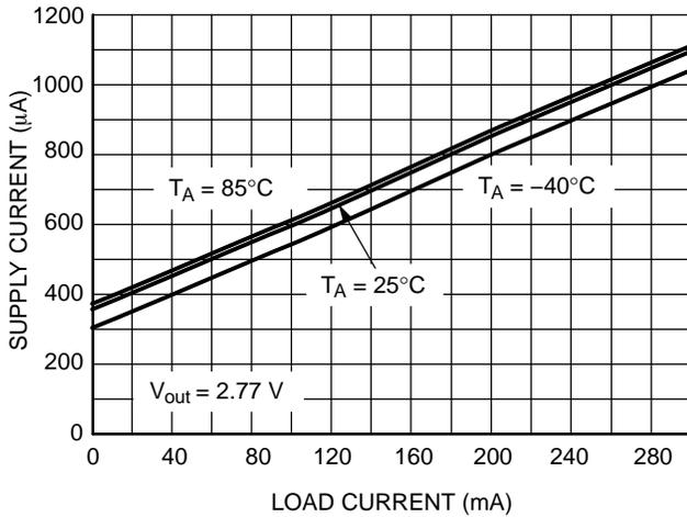
**Figure 3. Supply Current vs. Load Current**
