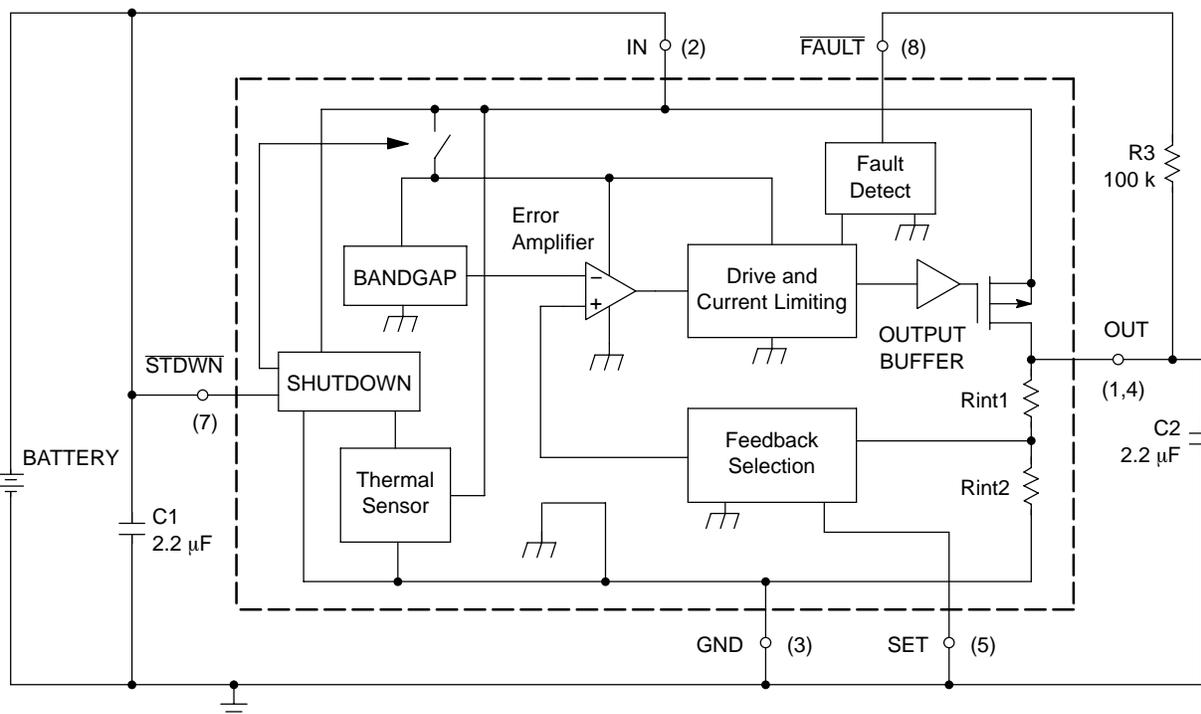
Figure 16. Application for 2.77 V Output Voltage
