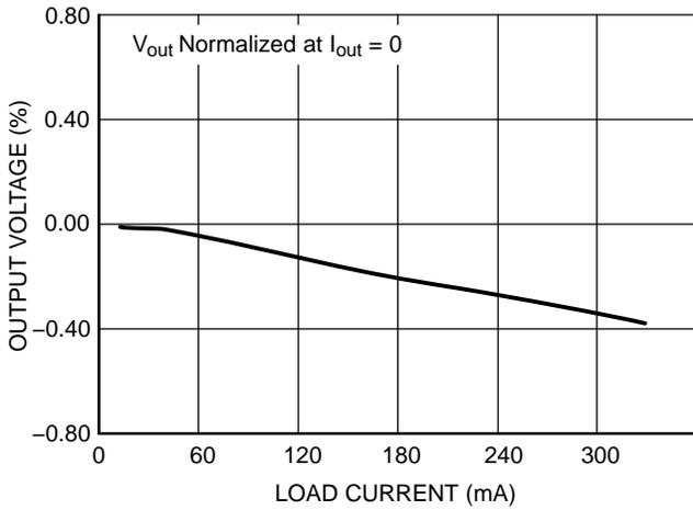
**Figure 1. Normalized Output Voltage vs. Load Current**
