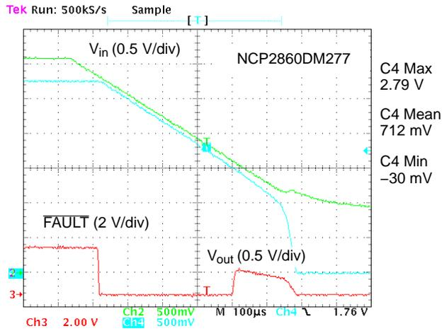
Figure 11. Power-Down Response ( $I_{load} = 100\text{ mA}$ )
