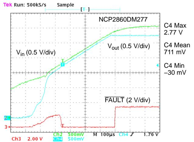
Figure 12. Power-Up Response ( $I_{load} = 100\text{ mA}$ )
