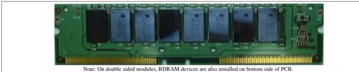
Figure 1: RIMM Module shown with heat spreader removed
