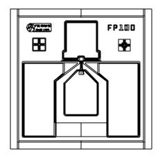
DIE SIZE: 16.5 x 16.5 mils (420 x 420 μm) DIE THICKNESS: 3.9 mils (100 μm typ.) BONDING PADS: 3.3 x 3.5 mils (85 x 90 μm typ.)
