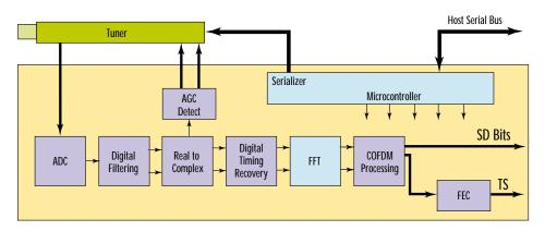
The L64782 is a highly integrated device that contains both digital timing and frequency loops. No external components are needed to operate the demodulation and only a low cost crystal is required.
