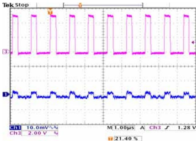
**Figure 11** – Switching Waveforms: PWM Mode
