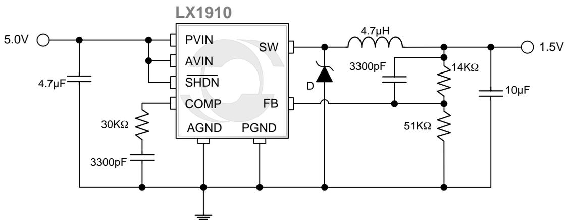
**Figure 3 – Circuit for 1.5V Output Voltage**
