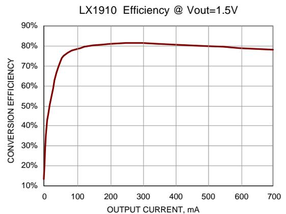
**Figure 1 – LX1910 Circuit Topology and Typical Efficiency Performance**
