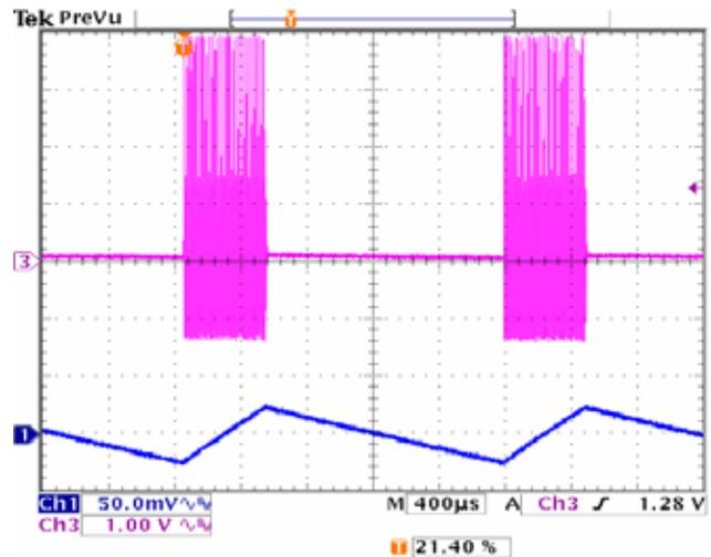
**Figure 10** – Switching Waveforms: PFM Mode
