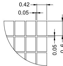
The tolerance unless classified  $\pm 0.3\text{mm}$
