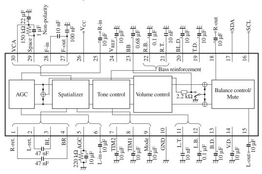
• Application circuit example of obtaining L+R output instead of bass reinforcement
