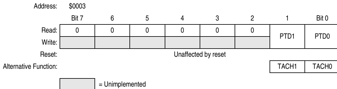
Figure 12-10. Port D Data Register (PTD)
