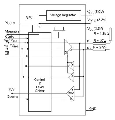
Figure 1. Logic Diagram
