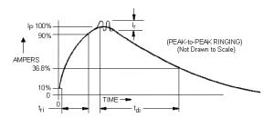
Figure 4. HBM Current Waveform
