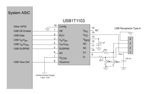
Figure 7. Downstream Connection in Normal Mode with Differential Outputs
