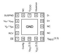
Figure 2. MLP16 GND Exposed Diepad (Bottom View)
