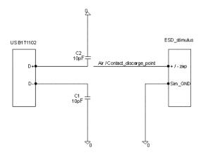
Figure 5. IEC 61000-4-2 ESD Test Model
