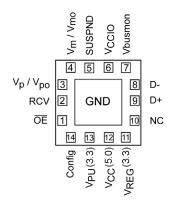
Figure 3. MLP14 GND Exposed Diepad (Bottom View)
