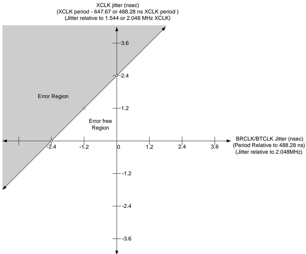
The BRCLK/BTCLK jitter is described as the worst case instantaneous peak jitter relative to a jitter-free BRCLK/BTCLK. The XCLK jitter is described as the worst case instantaneous peak jitter relative to a jitter-free XCLK. The jitter for both XCLK and BRCLK/BTCLK are described as positive and negative peak jitter in nanoseconds (ns). Positive peak jitter increases the instantaneous period while negative peak jitter shortens the instantaneous period.
