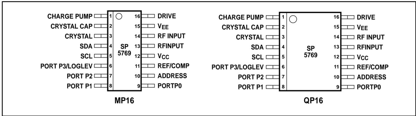
Figure 2 - Pin connections - top view
