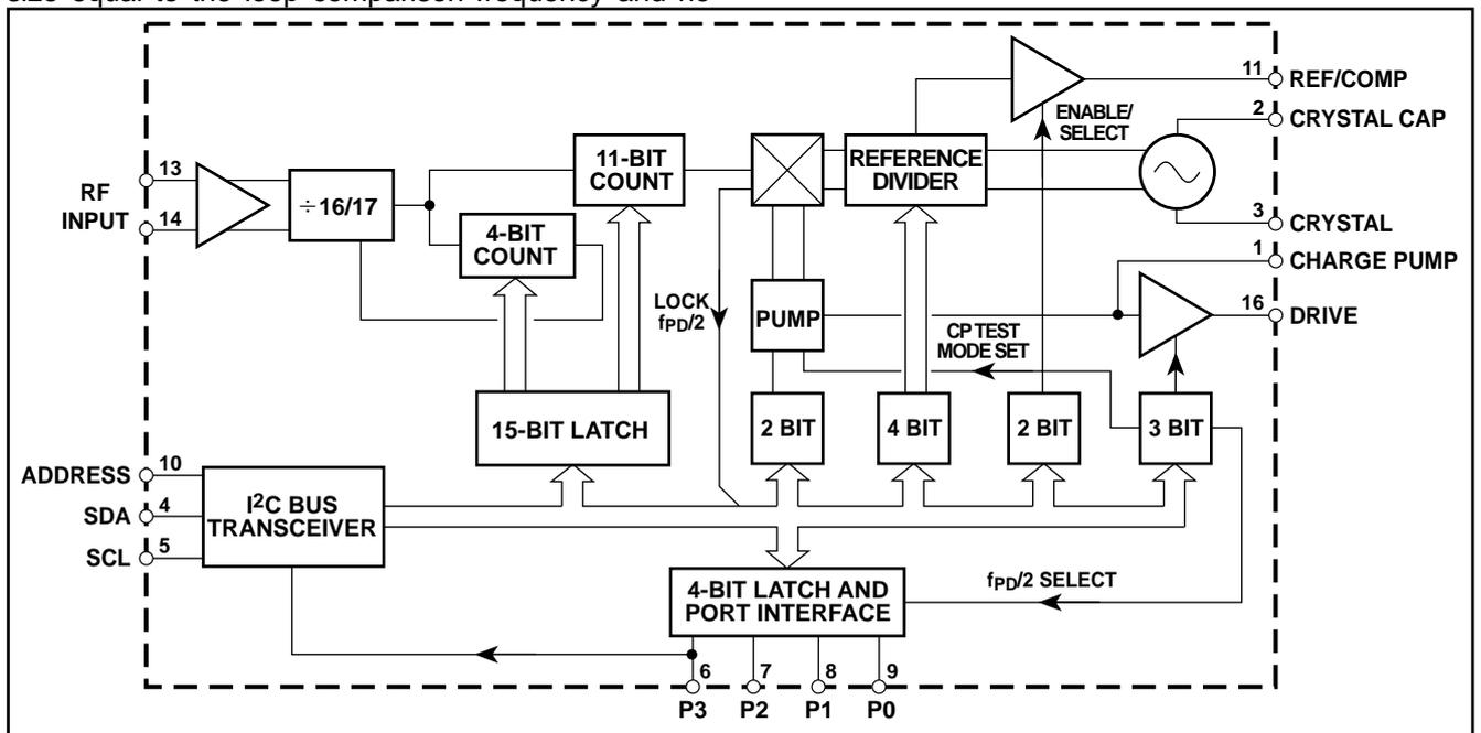
Figure 1 - SP5769 Block Diagram
