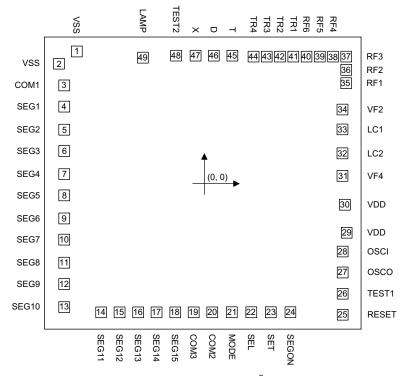
Chip size:  $2680 \times 2460 \ (\mu m)^2$ Chip thickness=12 mil
