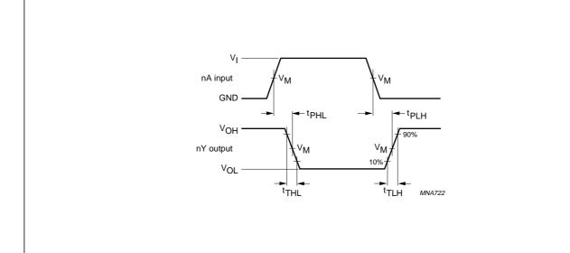
For HC3G:  $V_M$  = 50%;  $V_I$  = GND to  $V_{CC}$ . For HCT3G:  $V_M$  = 1.3 V;  $V_I$  = GND to 3.0 V.
