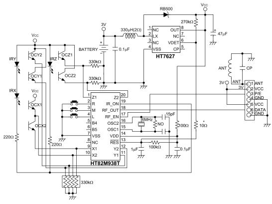
Note: \*  $10\Omega$  is placed if HT7627 is used to reset HT82M938T
